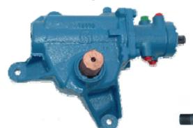
5696067A has 9/16 ports & uses one Saginaw cylinders. 5696067B has 11/16 ports & uses two Saginaw cylinders.
