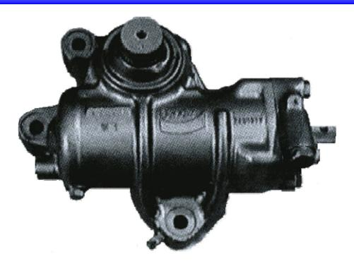
The casting number on the Bendix steering gear is the part number and of course, we always like to know the year/make/model of the vehicle to insure the correct gear.
