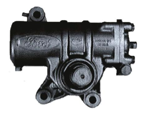
The casting number on the Bendix steering gear is the part number and of course, we always like to know the year/make/model of the vehicle to insure the correct gear.
