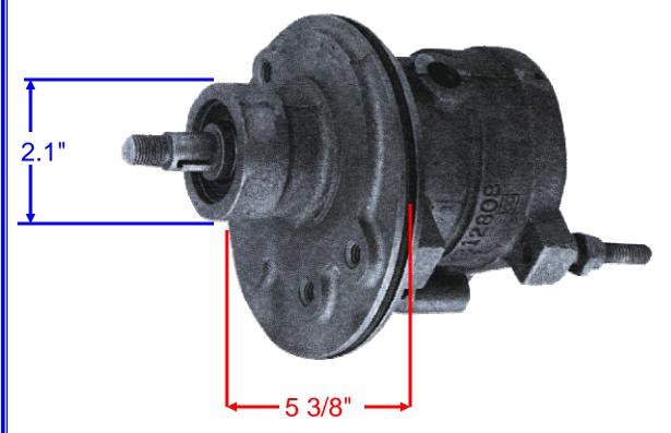
There are THREE belt driven Saginaw pumps. Two are BIG BEARING and the third is a BUSHING type. The out side diameter is the same on all three pumps - 5 3/8".
